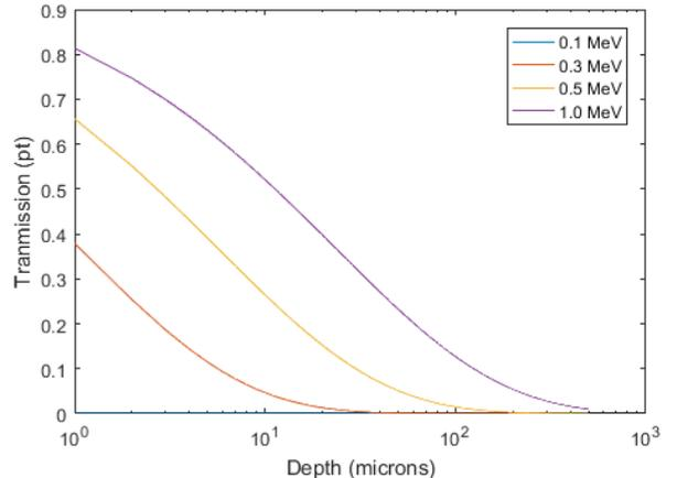
**Figure(1)** shows the transmission through a tungsten sphere at a specified depth - this provides the blurring depth for different energy x-rays. This corresponds to the 1D attenuation for path lengths through a tungsten carbide "sphere" with a radius of curvature of 0.5m. [7]
