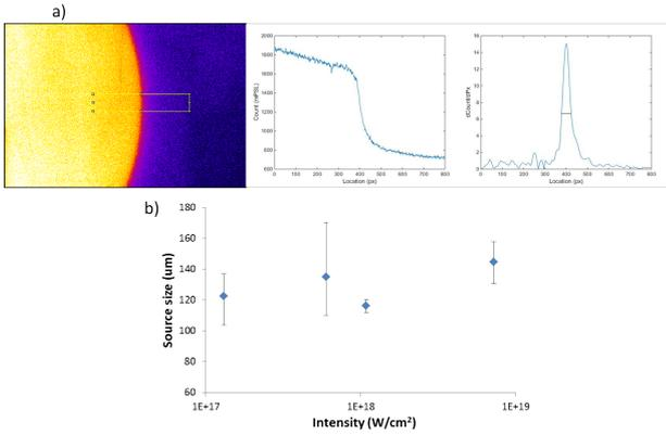
**Figure(2)** a) an example image cast by the penumbral aperture, with the two subsequent inset graphs being a lineout and the gradient showing the source size b) shows the results from the defocus scan on 100μm tantalum, error bars shown account for the asymmetry of the source and variance in the source further corrections can be made by accounting for the point spread function (PSF) of the filter layers.
