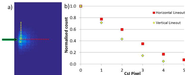
**Figure(4)** a) Image of the CsI scintillator leaking light across numerous pixels, b) Horizontal and vertical normalised line out showing a 75% transmission from one to the next
